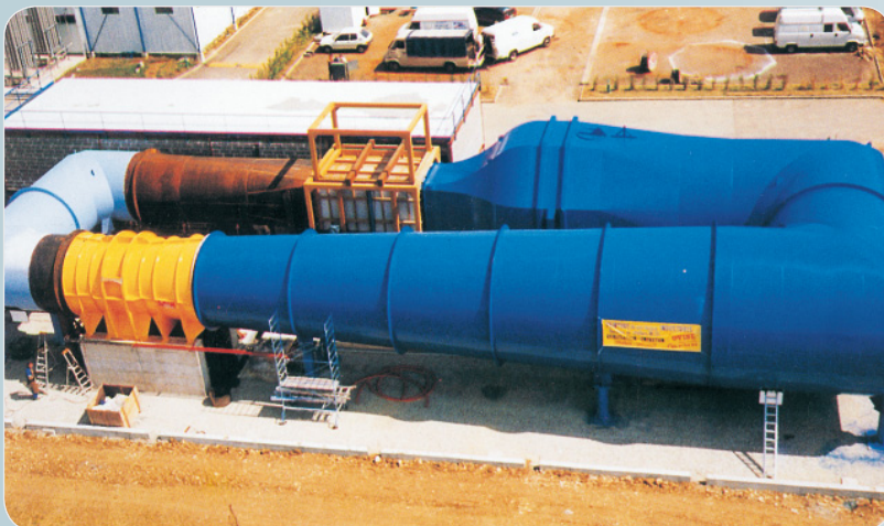
104-tonne wind tunnel for testing Formula 1 car aerodynamics (LIGIER)
