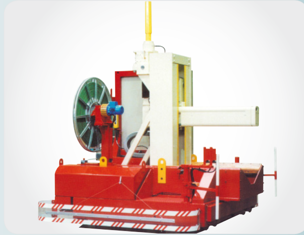
Automatic truck for transferring and loading 11-tonne steel coils. (ARCELOR MITTAL)
