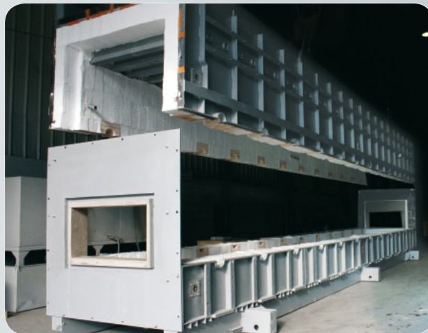
Industrial furnace with refractory fibre lining (SERMAS).
