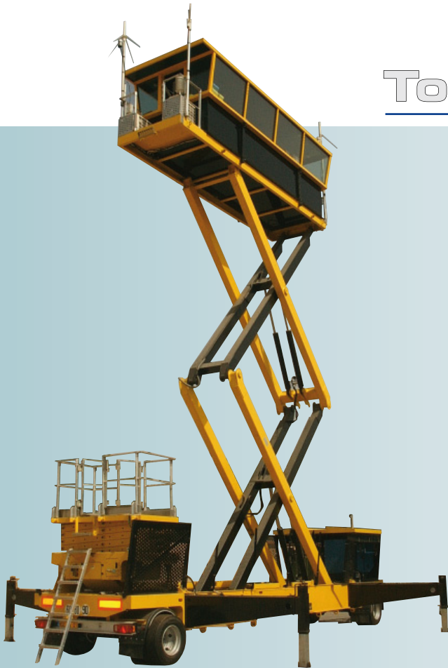
Mobile air control tower with access pod (TWIST)
