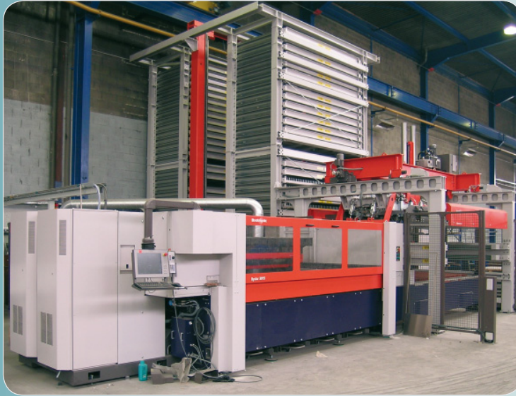
Laser Machine with its storage unit (capacity of 40 tonnes of sheet metal)
